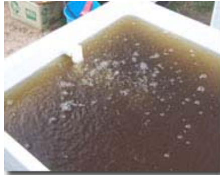
LEFT:- The water comes into the tank via a venturi tube which sucks air into the water creating an excellent source of aeration for the fish. The air bubbles can be seen rising in the water.
