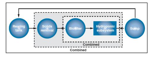
Figure 8 A typical arrangement of aquaponics system components (Rakocy, Masser & Losordo 2006)
