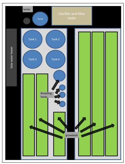
Figure 63 A potential layout for a near-ideal aquaponics system (approximately drawn to scale)
